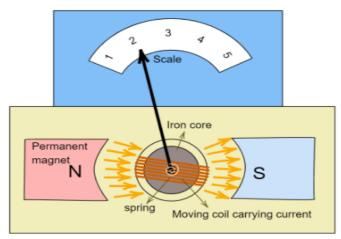
Front view of a Moving Coil Galvanometer
